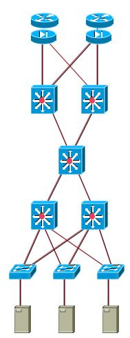
*Perimeter*: device integrity, stateful firewall, NIDS, uRPF and spoof mitigation, L3 filtering, DDoS mitigation, URL filtering, CAR
