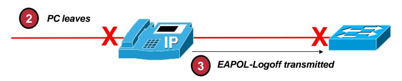
If an end-user disconnects, an IP Phone transmits an EAPOL-Logoff frame to the switch.
