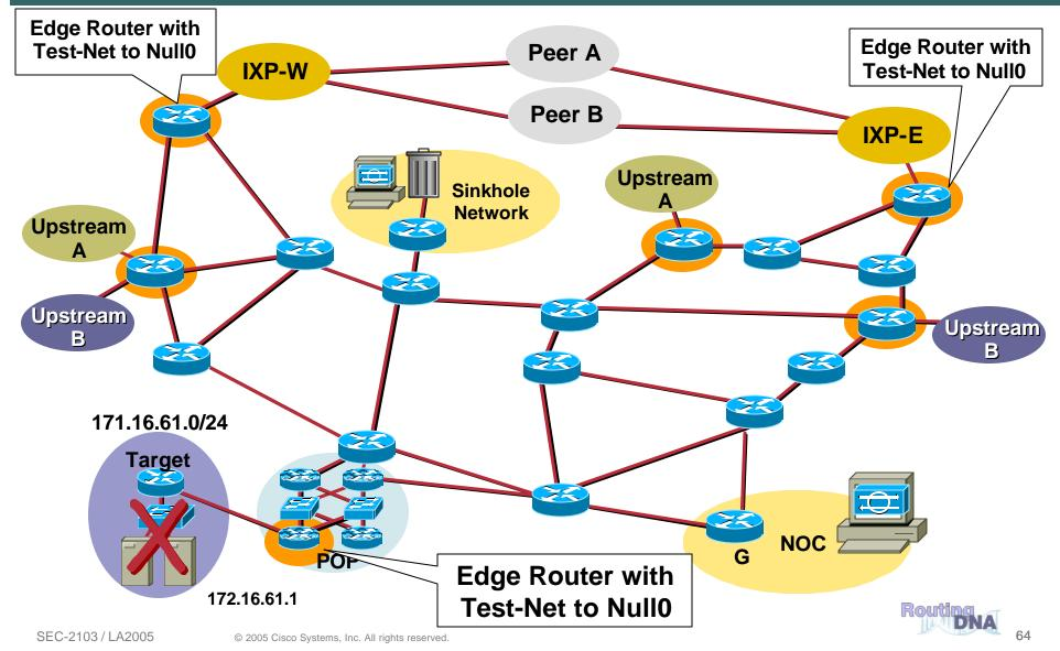
The trigger router is the device that will inject the iBGP announcement into the ISP's Network
