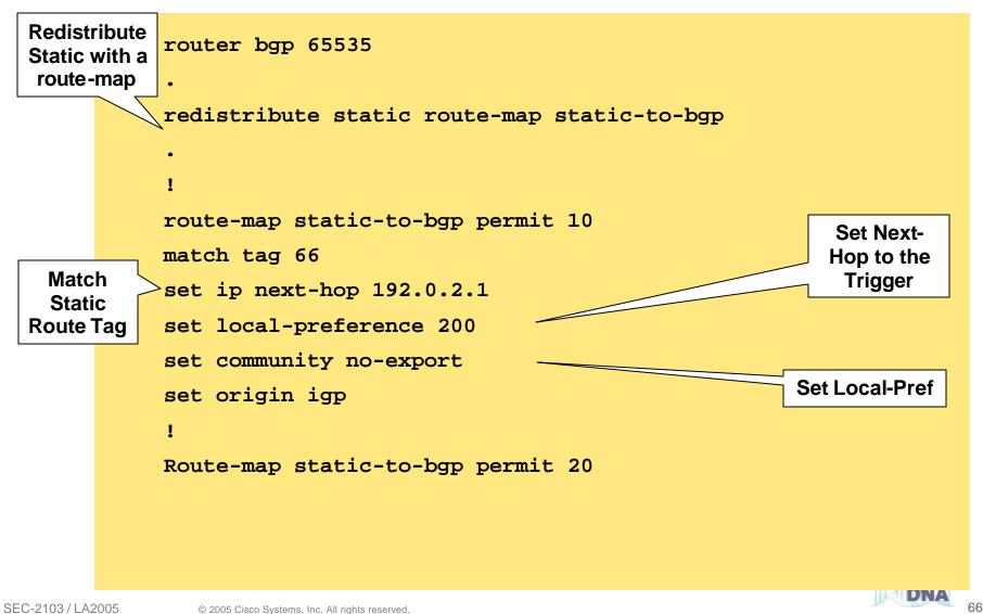
Add a static route to the destination to be blackholed; the static is added with the "tag 66" to keep it separate from other statics on the router
